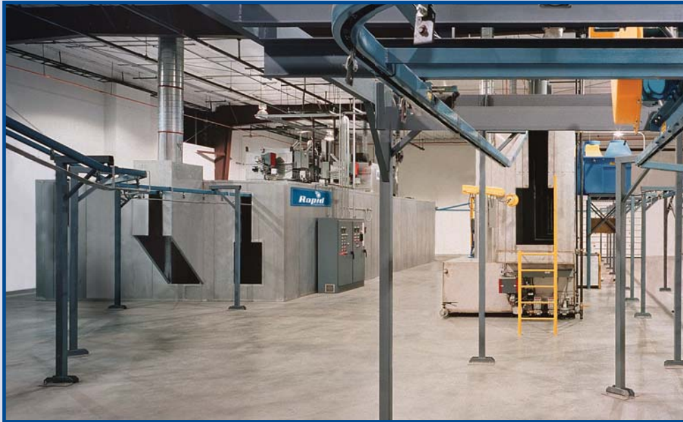
A typical RAPID™ Finishing System with five-stage washer, dry-off oven, cure oven and conveyor.
